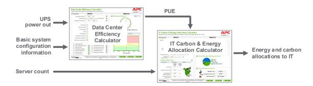
The user provides basic information about the configuration of the data center and the server count, along with current readings of UPS load power taken from the UPS (this is one of the only power readings that is available in almost any data center). The software tools prompt for the relevant information, information which any data center or IT professional should be able to obtain, or determine by a simple walk-through.
