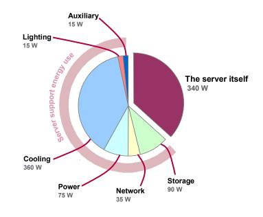
In this case, even though the actual power drawn by the typical server is 340 W, the total power allocated to the server is a much larger 930 W.
