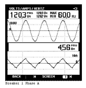
This waveform is from circuit breaker (CB) 1 - Phase A. The current waveform represents the positive effect of the load diversity. In this case the relative high ratio of linear to nonlinear load is seen in the waveform. It also can be seen in the system power factor and THD measurements. When loads with differing characteristics are combined in a single circuit
