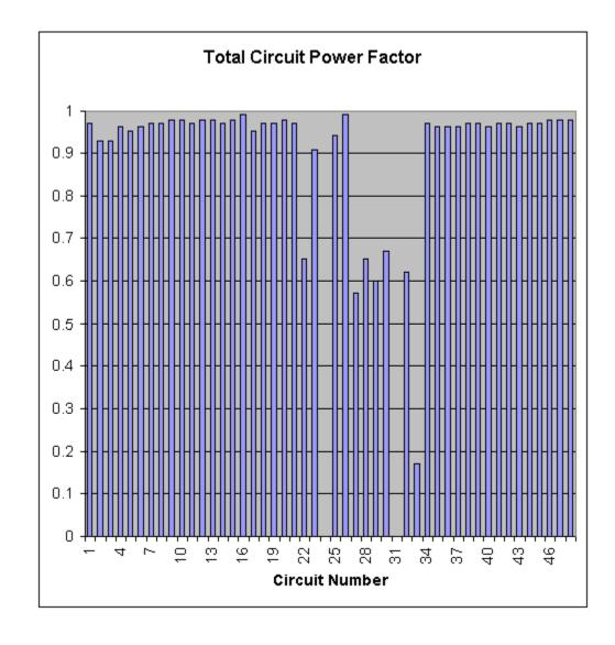
This chart shows the total power factor of all branches. We can see that the majority load is .95 or better and also has same pattern as the previous charts, i.e., lowest power factor is the lightest loaded circuits. The overall power factor of the system will be higher than the average of these power factors, because the data shows that the circuits with low power factor also have low current, and therefore the circuits with low power factor make a low contribution to the total reactive power.
