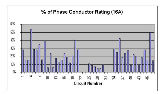
This chart shows the branch circuit loads relative to the 16A conductor rating for each branch. Once again there is no balance indicated for any of the three-phase multi-wire circuits and the highest % load is ~ 55% on branch # 4 (CB #2- A Phase). The majority circuit loading is under 30% of the conductor rating.
