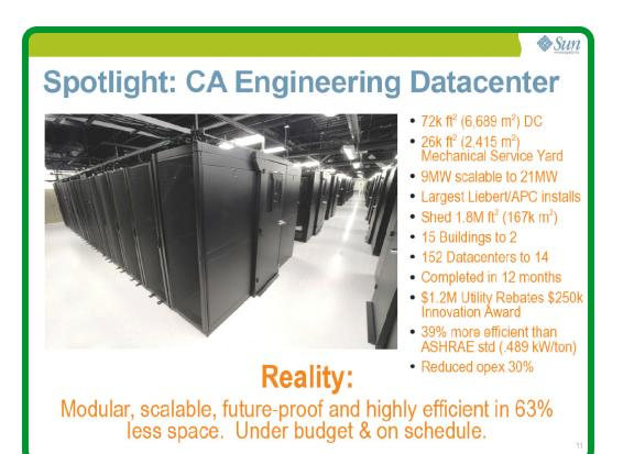
In the example of **Figure 2**, a high density pod based approach was used in a new data center as part of a massive consolidation project of 152 data centers to 14 data centers. This project resulted in a PUE of less than 1.3. The pod approach simplified the design and accelerated the timeline of the project which was completed in 12 months.
